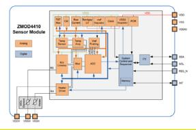
**Silicon-based Digital Gas Sensor Platform**
