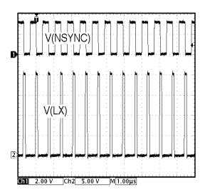
FIGURE 19. LX SYNCHRONIZATION WITH f(SYNC) = 1.4MHz
