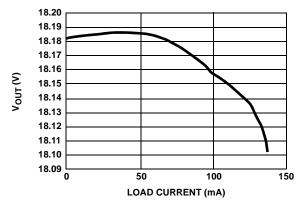
FIGURE 11. LOAD REGULATION ( $V_{IN} = 3.6V$ )
