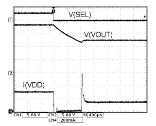
FIGURE 9. 18V->12V TRANSITION (V<sub>DD</sub> = 3.6V, R<sub>L</sub> = 360 $\Omega$ )
