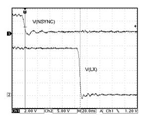
FIGURE 17. NSYNC TO LX SYNCHRONIZATION DELAY
