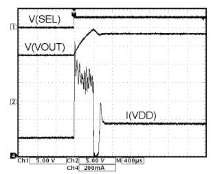
FIGURE 8. 12V->18V TRANSITION (V<sub>DD</sub> = 3.6V, R<sub>L</sub> = 360 $\Omega$ )
