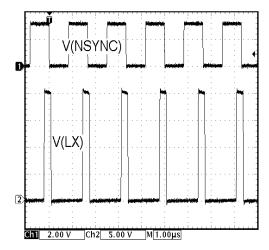
FIGURE 18. LX SYNCHRONIZATION WITH f(SYNC) = 600kHz
