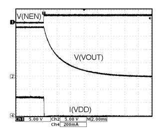
FIGURE 10. SHUT DOWN @ SEL = 1 (V $_{DD}$  = 3.6V, R $_{L}$  = 360  $\!\Omega)$
