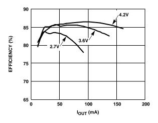
FIGURE 4. EFFICIENCY vs I<sub>OUT</sub> ( $V_{OUT}$  = 12.6V) L = 6.8 $\mu$ H (TDK RLF7030) C = 6.6 $\mu$ F
