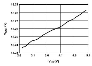
FIGURE 12. LINE REGULATION (I<sub>OUT</sub> = 30mA)
