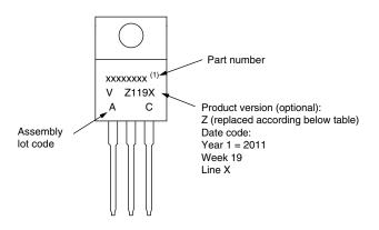
Example: This is a xxxxxxxx (1) with assembly lot code AC, assembled on WW 19, 2011 in the assembly line "X"
