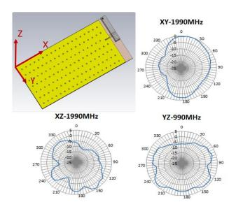
FIGURE 6.2 RADIATION PATTERN OF ATNENNA AT 1990MHZ IN FREE SPACE
