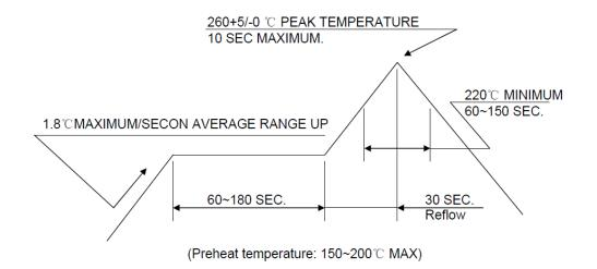
FIGURE 7.1 RECOMMENDED SMT REFLOW PROFILE
