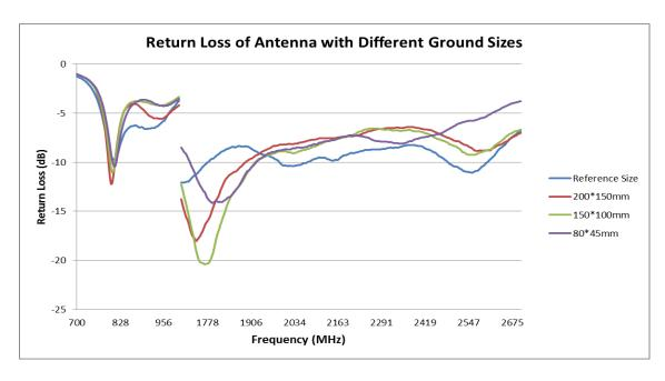
FIGURE 4.5.1 RETURN LOSS COMPARISON AT 790-960MHZ and 1.7-2.7GHz BAND OF ANTENNA MOUNTED ON DIFFERENT SIZE GROUND
