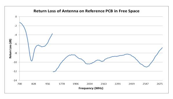
FIGURE 2.2 RETURN LOSS OF ANTENNA AT 790-960MHZ AND 1.7-2.7GHZ BAND AT REFERENCE LOCATION IN FREE SPACE
