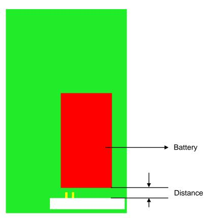
FIGURE 4.2 SIMULATED CONDITION: BATTERY FIXED ON REFERENCE PCB
