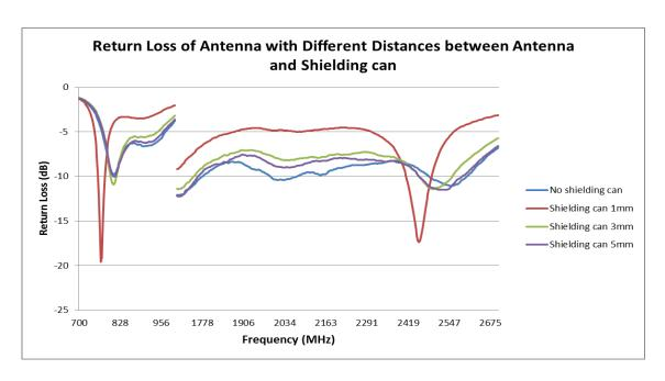
FIGURE 4.1.1 RETURN LOSS COMPARISON AT 790-960MHz AND 1.7-2.7GHZ BAND OF DIFFERENT SHIELDING CAN DISTANCE FROM ANTENNA
