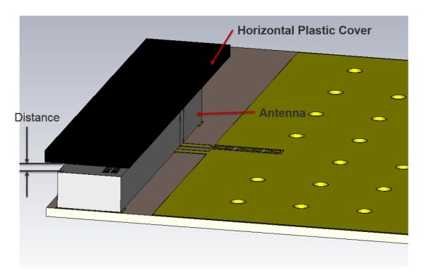
FIGURE 4.4 DIFFERENT DISTANCE BETWEEN HORIZONTAL PLASTIC COVER AND ANTENNA
