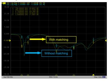
FIGURE 5.5 RETURN LOSS OF ANTENNA WITH AND WITHOUT MATCHING ON 130\*60MM GROUND
