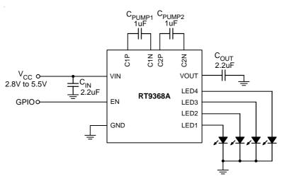
Figure 1. For 4-WLEDs Application Circuit
