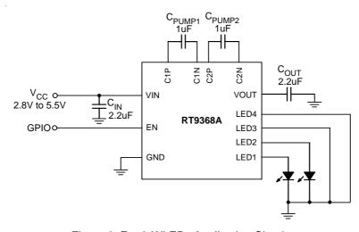
Figure 3. For 2-WLEDs Application Circuit
