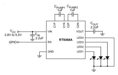
Figure 2. For 3-WLEDs Application Circuit
